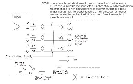
Figure 23: Command Connector Encoder Output Wiring
